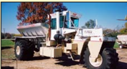
1997 Tyler 3330 Cat, Allison World Auto. New Leader L2020GT 304 Stainless Steel Spinner Box with Belt over Chain Conveyor and Raven Controller.
