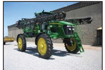
JD 4830: 1000g SS Tank, 100' SS Booms on 20", Dual Flow Meters, Eductor, Hyd Tread Adj., Air System, Auto Level System, Traction Control, Dlx Cab, HID Lights, Return to Ht., 380/80R46, Warranty Until April 2011, 1050 hrs. $190,000.00 (wf)
