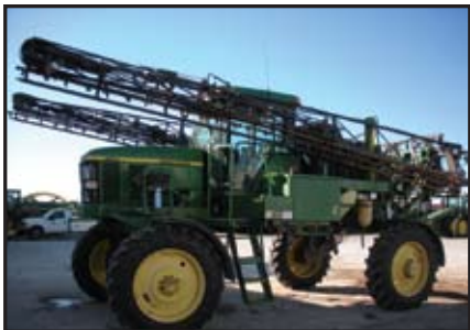
JD 4700: 750g Poly Tank, 90' Boom on 20" Spacing, Hydraulic Tread Adjust, Rinse Tank, Eductor, Below Horizontal Tilt Cyl, 2668 hrs. $75,000.00 (am)
