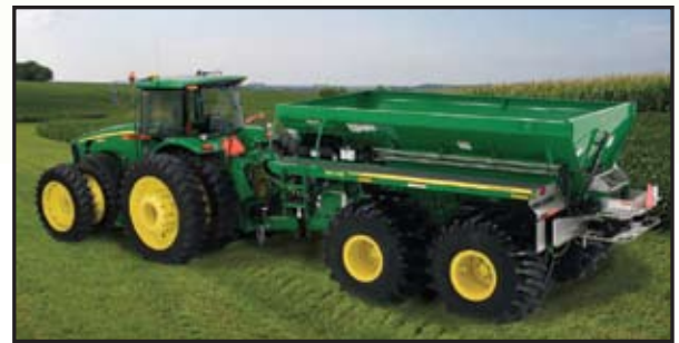
JD DN345 Drawn Dry Box Spinner Spreader made to handle 345 cu ft of Fertilizer or Lime
