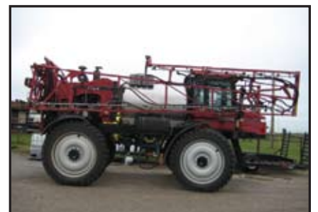
Case SPX 3310: 1000g SS Tank, 90' SS Booms on 20", Foamer, RH & LH Fence Row Nozzles, 380/85R46 Tires, Hyd Tread Adj., 3" Q.F., Raven SCS 4600 Controller, Raven Auto Steer System, Traction Assist, 1250 hrs. $138,500.00 (cl)
