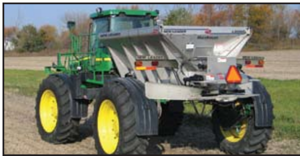
JD 4900 325 Hp w/ choice of New Leader G4 200 cu ft or 300 cu ft spreader boxes
