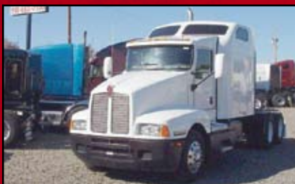
2005 KENWORTH T600 , 72" Aerodyne Sleeper, C-15 Caterpillar Engine 475 HP, Diesel, 484,500 Miles, 10 SPD OD, Engine Brake, 8 Bag Air Ride Susp, 3.36 Ratio, 22.5LP Tires, Alum/Steel Wheels, 230" WB, Tandem Axle, 12,000 # FA, 40,000 # RA, Stk #1780
