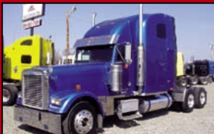
2001 FREIGHTLINER FLD13264T-CLASSICAL XL , 70" Condo Sleeper; 12.7 Detroit Engine 470 hp; Diesel; 958,961 Miles; 10 Spd OD; Engine Brake; Air Ride Suspension; 3.55 Ratio; 22.5LP Tires; Aluminum Wheels; 259" WB; Tandem Axle; 12,000 # FA; 40,000 # RA. Stk #1806. US $19,900
